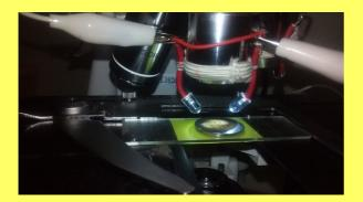
With the help of a battery box and two Cayman wires and I turn on the LEDs with a switch. Shown below is the system for only one for the two objectives.
