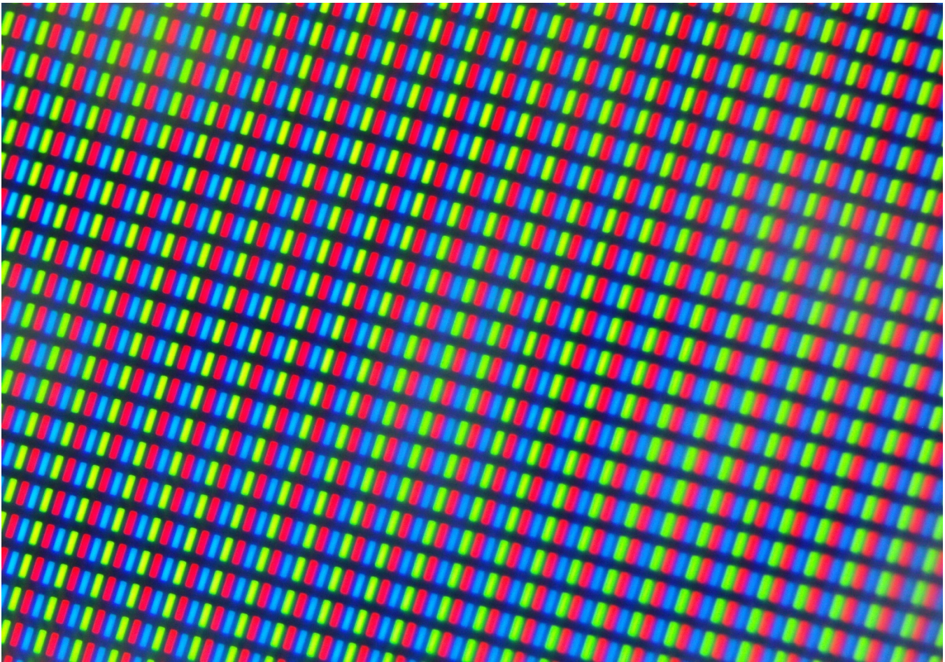
White part on the screen 4x, it is appreciated that to show the white color, the three components are present.
