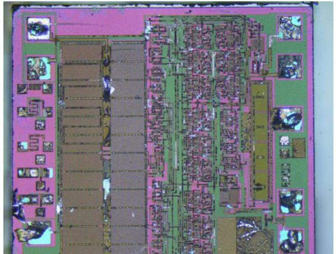
Illustration 6: Quartz watch IC after a second heating and a further 3 minutes of ultrasonic cleaning
