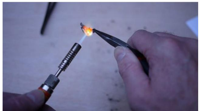
Different devices have different characteristics and some separate from the packaging easily, some take a bit more work. Now and again there seem to be coatings on dies and I may have to burn this off with a second heating with the torch. If there's a lot of debris on the die after removal from the package I use an ultrasonic cleaner to remove it. I use plain water as the cleaning fluid and run the cleaner for about 3 minutes.
