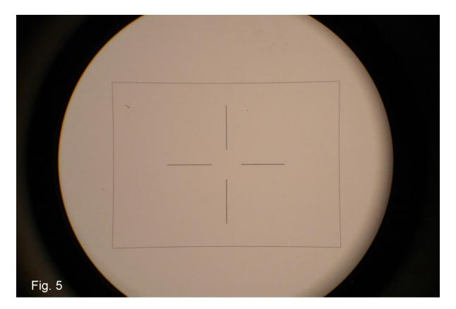
Fig. 5 shows the view through the eyepiece with the reticle installed.
