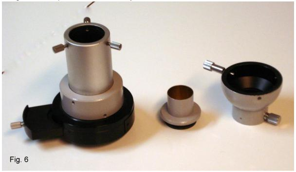
Fig. 6 shows the vertical tube with the removable top part. This can be exchanged for a Cmount adapter for a video camera (see Fig. 14) and an optional adapter for other accessories (on the right). On the Leitz Periplan eyepiece (Fig. 7) you will notice three small white patches. These are soft spacers to prevent the camera objective from being scratched when the eyepiece is screwed onto the digital camera.
