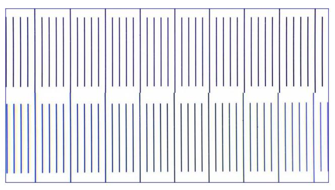
Comparison between eyepiece projection with a hybrid eyepiece (top) and a raised Kpl W10x eyepiece (bottom). Chromatic aberration is clearly visible with the normal eyepiece. Objective: CZ Plan 25/0.45.
