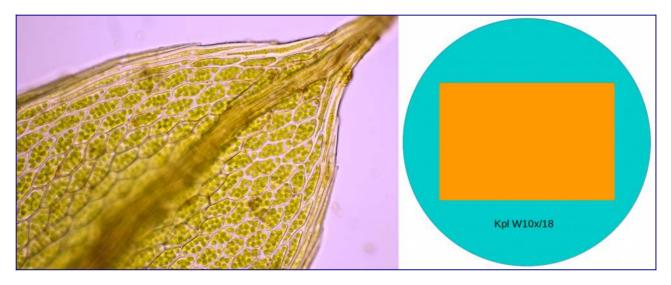
Left: a moss photographed with a Zeiss Planapo 25/0.65 and hybrid Kpl8x-Kpl10x eyepiece. Right: The orange rectangle indicates the part of the microscopic field of view that is photographed using this eyepiece and a Canon 600D camera. The circle refers to an eyepiece with a field number of 18, such as a Zeiss Kpl W10x/18 eyepiece.
