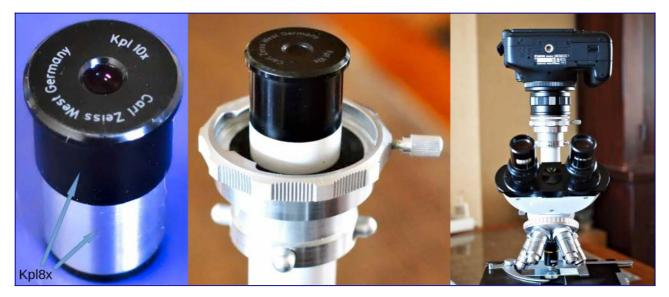
Combination of a Zeiss Kpl8x and Kpl10x eyepiece in use as a projection eyepiece with the Zeiss Standard and a Canon 600D camera. The field lens and the eye lens of a Kpl10x eyepiece were screwed onto a Kpl8x body.
