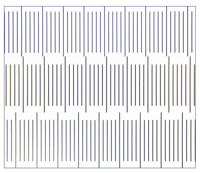
Stage micrometer photographed, from top to bottom, with Carl Zeiss Plan 25/0.45, Neofluar 25/0.60 and Planapo 25/0.65. Projection with hybrid Kpl8x-Kpl10x eyepiece.
