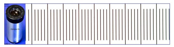
Hybrid eyepiece composed of 3 different eyepieces. Right: Stage micrometer photographed with this eyepiece and a Leitz NPL Fluotar 25/0.55 objective on the Leitz Laborlux-12.
