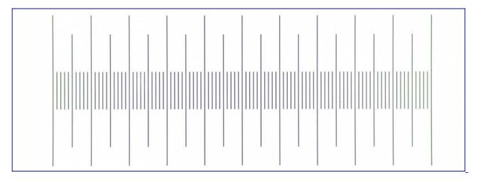
Stage micrometer photographed with a Zeiss Plan 10/0.25. Eyepiece projection with a hybrid Kpl8x-Kpl10x eyepiece.
