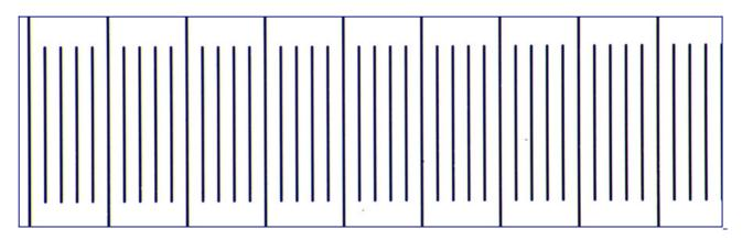
Stage micrometer photographed with 37 mm Olympus Plan 20/0.40 objective. Here, an Olympus FK2.5x projective was used in combination with the Olympus OM-Mount Photomicro' Adapter L. It is clear that a smaller part of the field of view is captured compared to the hybrid eyepiece. Camera: Canon 600D.
