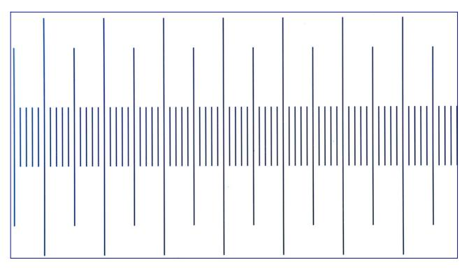
Stage micrometer photographed with a 37 mm Olympus Plan 20/0.40 objective and hybrid eyepiece. Camera: Canon 600D.
