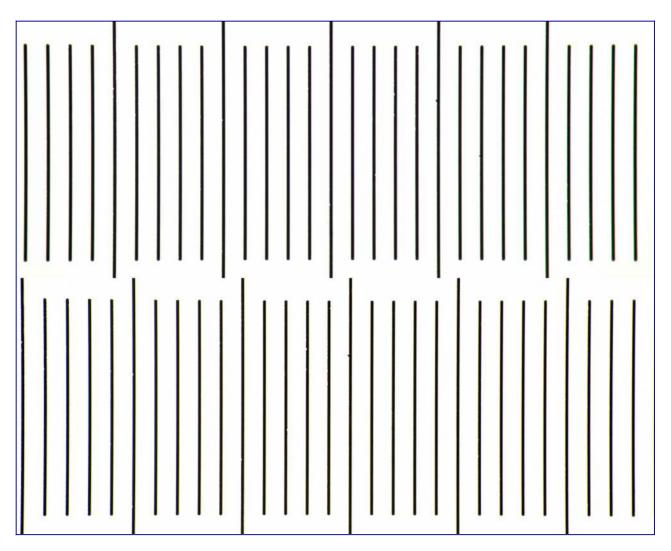
Stage micrometer photographed with Zeiss Plan 40/0.65 (top) and Zeiss Planapo 40/1.0 (bottom). Projection with hybrid Kpl8x-Kpl10x eyepiece.
