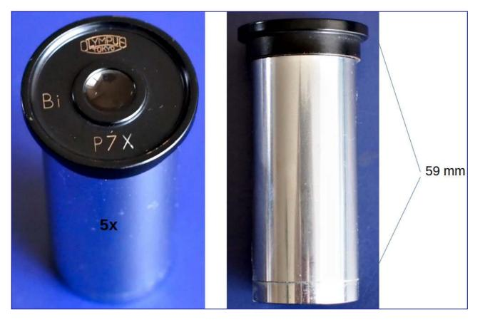
Hybrid eyepiece consisting of the lower part of an unbranded 5x eyepiece and the eye lens of an Olympus P7x eyepiece.
