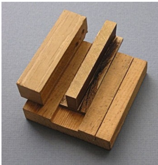
Figure 7. Three-piece wooden jig for bending clips. Dimensions not marked are flexible. The T-shaped piece represents the thickness and width of (slide + cover glass). The trough is slightly wider so the clip and T-shaped piece fit. The 8 mm depth of the saw kerf is (side height + flange width). Aluminum blanks are cut (27 + 8 + 8) mm = 43 mm wide. The plain block is a burnisher for creasing folds.
