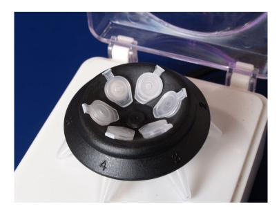
The rotor holds six 1.5 milliliter vials. You can centrifuge two or six vials at a time since the weight has to be evenly balanced. All of the vials must have equal amounts of fluid to maintain balance. If two vials are used they must be in positions opposite of each other.
