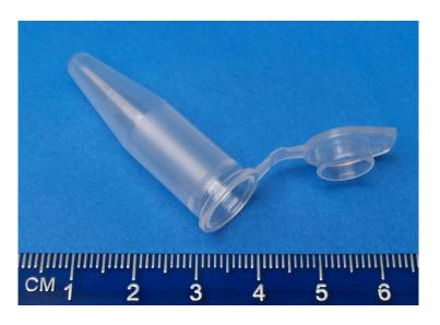
The 1.5 milliliter vials have a snap cap to prevent aerosols being created that would occur with an uncapped vial due to the Venturi Effect.
