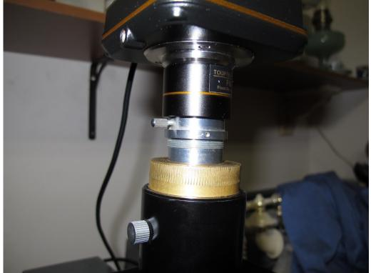
Generic C mount image reduction lens systems seem very difficult to locate, but fortunately the provided system works fine as long as one can find a way to get it at the right distance from the
