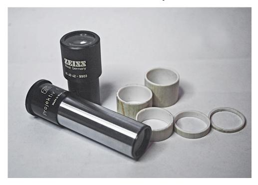
The Zeiss Projektiv f = 63mm (front), a Zeiss 10x KPL eyepiece (back) and several pieces of close fitting electrical PVC pipe cut to 2.5mm, 5mm, 10mm 15mm and 20mm used to *lift* the eyepiece by lengthening its shoulder. Varying the height over and above the initial *lift* that enables it to project a real image alters the magnification ratio.
