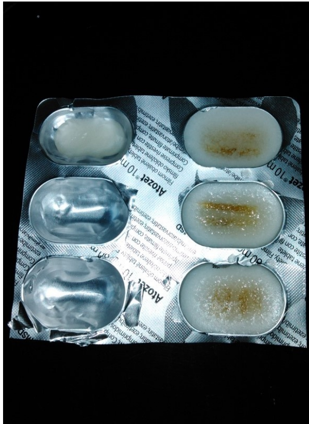
Molds with two pieces of stems placed in each, with the PEG almost completely solidified.
