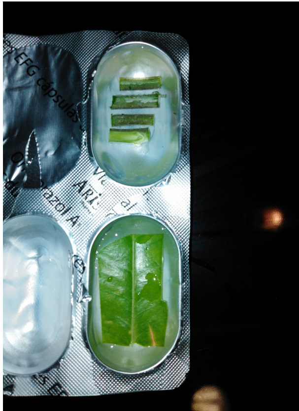
Placement of the material inside the blister with the PEG completely melted on the heating plate (glass ceramic).
