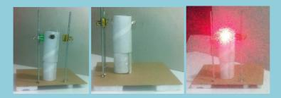
For holding the laser pointer I use the tube which I cut into two parts and made one slide inside the other so that this may be used to raise or lower the laser pointer as needed, here is a picture of it:
