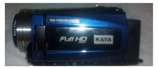
It is said that the NIR spectrum is a kind of lighting that passes almost unchanged from some types of media to another. That property allows NIR lighting to be used to reveal hidden details in some objects when the proper equipment is used as in the case of a camera whose NIR cut filter has been removed or that is mechanically removed by clicking a button as in the case of my camera.
