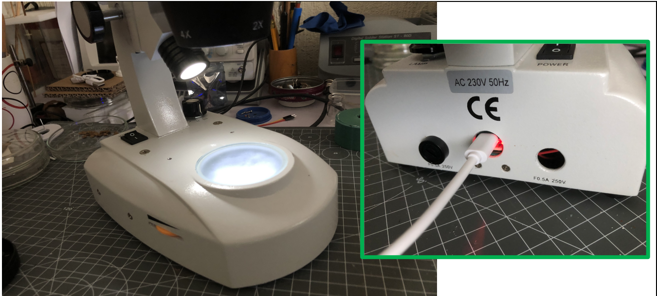
Figure 3: The refurbished microscope retains its epi-illumination feature. While the potentiometer offers some dimming capabilities, it could benefit from further improvements. Its portability and the convenience of quickly recharging the internal power source is an excellent advantage.
