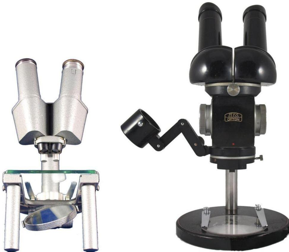
Figure 9. Leitz Greenough Side-by-Side with Zeiss Opton CMO Stereomicroscope, 1949, Inclusive 6x-10x-16x-25x-40x Magnification Changer like Zeiss Jena Citoplast, 1946.
