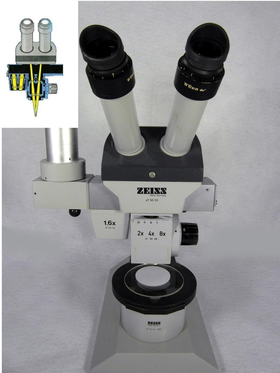
Figure 7. Zeiss Stemi DRC Greenough-style Body with Photo Port and Equipped with Changer D 2x-4x-8x, the 1.6x Objective Pair, and Transmitted-light Bright and Dark Field Illuminator, on an LO Stand, 1978. Zeiss Stemi DRC Light Paths with Permission of, Carl Zeiss Microscopy, LLC.
