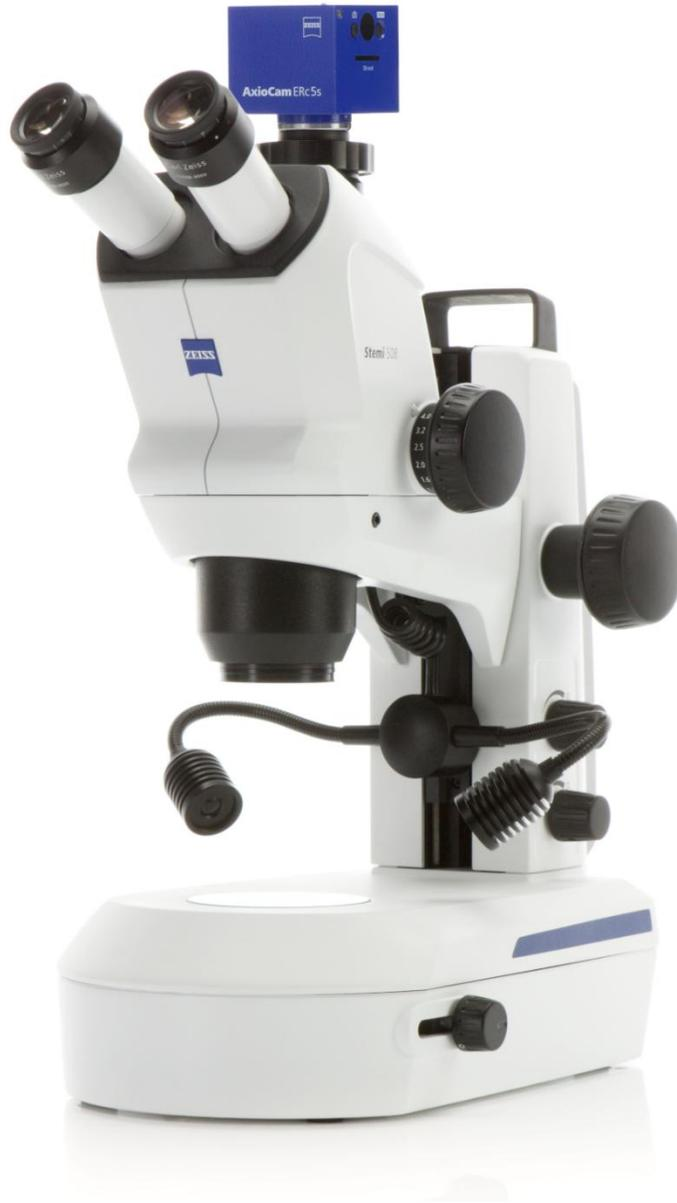
Figure 8. Today's Zeiss Stemi 508 doc Apochromatic Greenough Stereomicroscope with 8:1 Zoom, Equipped with AxioCam ERc5s Digital Camera, on K LAB Stand with Integrated LED Illumination. Courtesy of ZEISS Microscopy.
