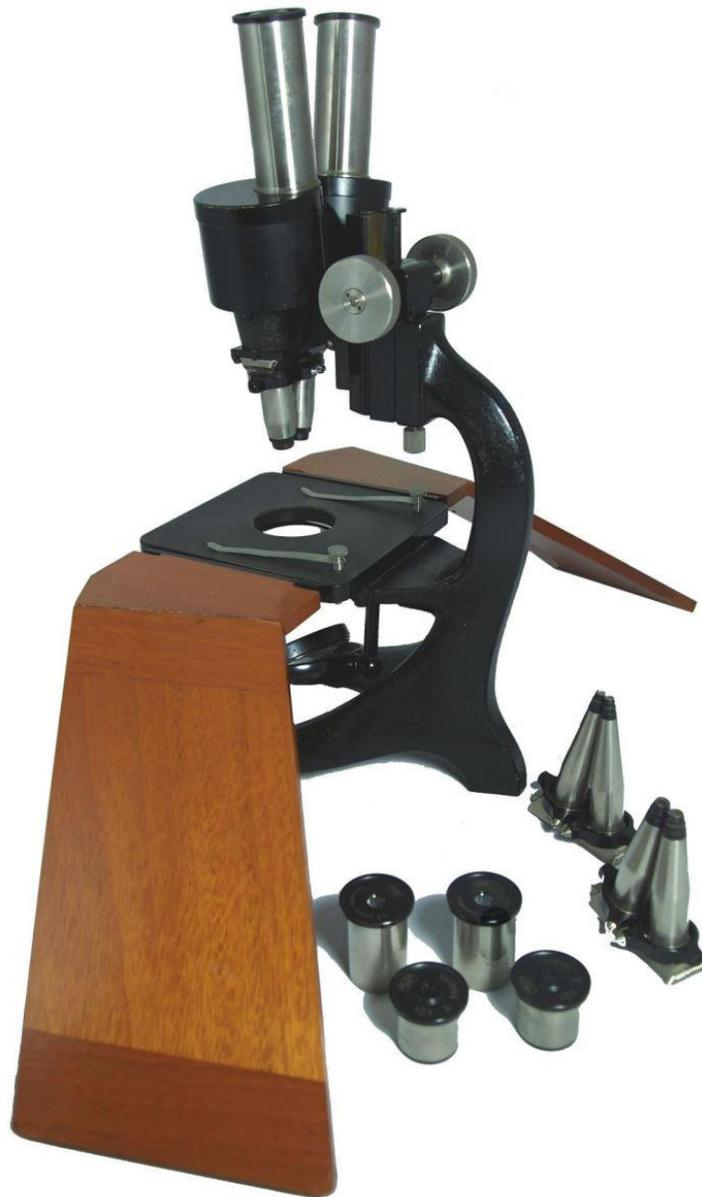
Figure 2. Zeiss Double Tube XA with Interchangeable Objective Pairs, 1923, Jena, Germany.
