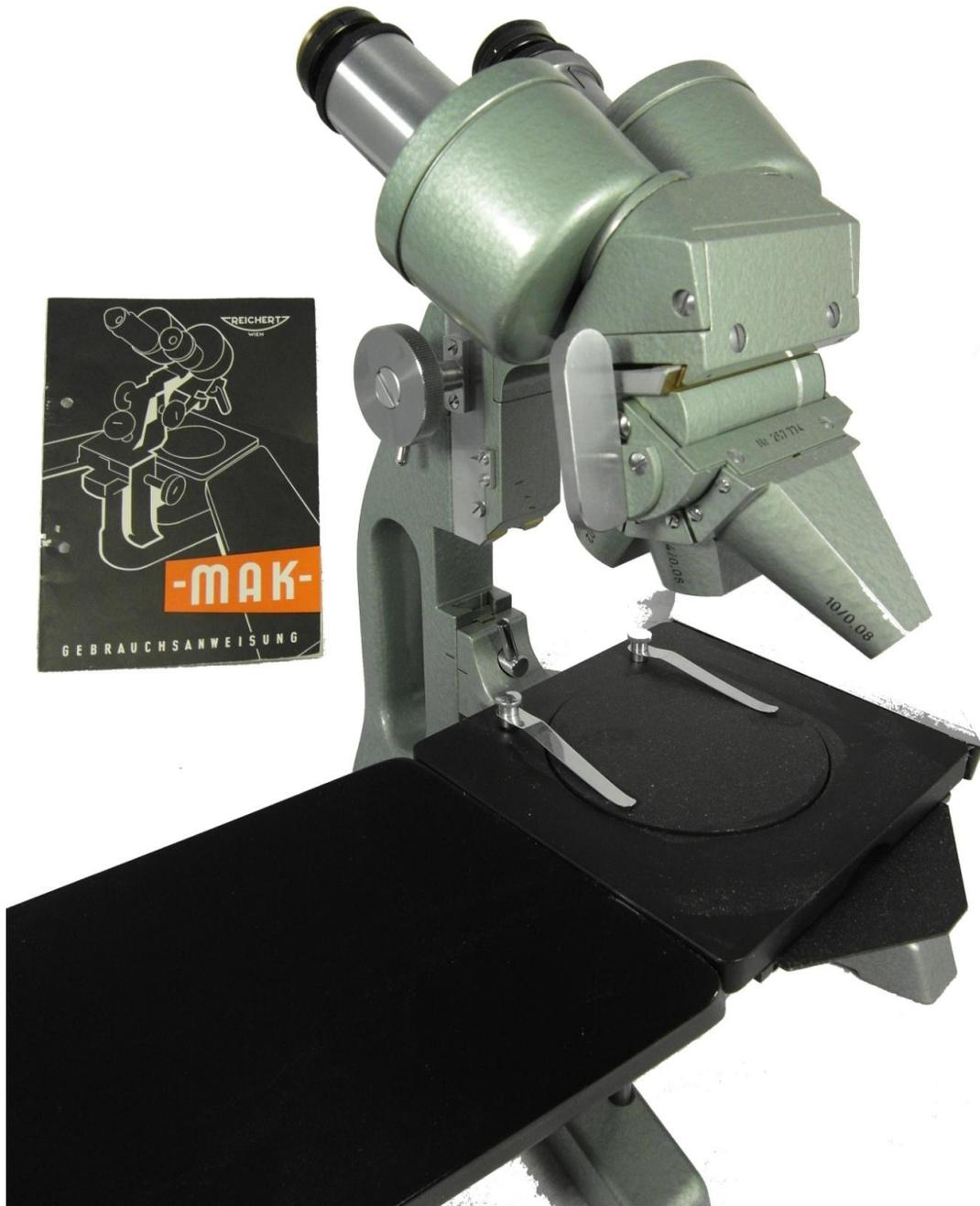
Figure 6. Jug Handle Reichert Greenough Stereomicroscope with Triple Objective Drum, ca. 1955, Wien, Austria.
