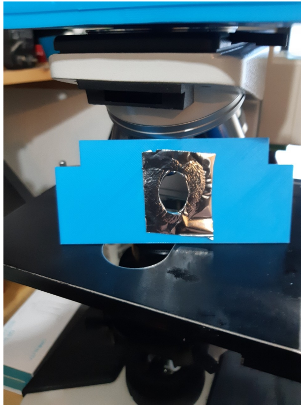
Ring of light seen at the base here before attaching the scope mounting ring
