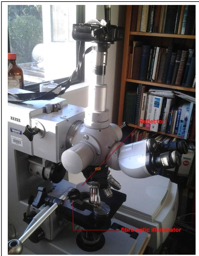
Fig 2. Low-power compound microscope Much smaller instruments than this one could do a good job.
