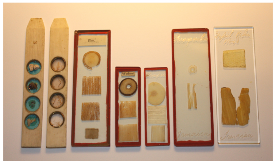
Figure 4. The list of microscope slides offered by Palmer in 1840. The photograph shows examples that correspond with Palmer's descriptions (please note that there are no indications that any of these examples was retained by Palmer). Left to right: ivory slide with four opaque objects, ivory slide with four transparent objects, double glass slide containing three sections of elm wood, two double glass slides containing three each sections of wood, double glass slide containing botanical objects (sarsaparilla), and a slide of sections of fossil wood. The double glass slides, sealed with red wax, are nowadays often attributed to Andrew Pritchard because he described their production in a 1847 book, and because such slides are occasionally found with Pritchard's name attached. However, there is no evidence that Pritchard actually made any of these slides, nor that he was the only retailer to have sold them. John Quekett, in his 'Treatise on the Use of the Microscope' stated that these slides were made by William Darker. A detailed biography of William Darker and his extensive involvement with early microscopy and optics is currently under production.
