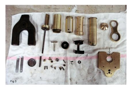
through the shimming plate and a slot in the prism shaft. The length of this slot limits the fine focus range. Turning the fine focus down lifts the outer body with the pin compressing the spring. In the illustration the hatched sections are the moving parts. I have not come across a similarly designed fine focus in my experience.
