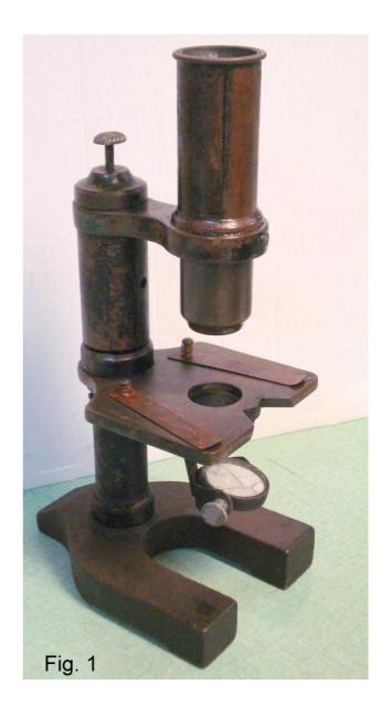
crudely made or had been tampered with subsequently. In any case it fits rather loosely into the outer part. There is a shimming plate, but it lacks the usual screws to press it against the shaft to reduce slack, nor can it be removed to underlay additional shimming because for some weird design it cannot be removed! This really puzzled me: the plate has an oblong recessed slot with a screw or bolt that prevents
