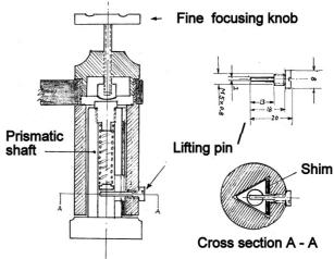
Schematic of focusing mechanism
