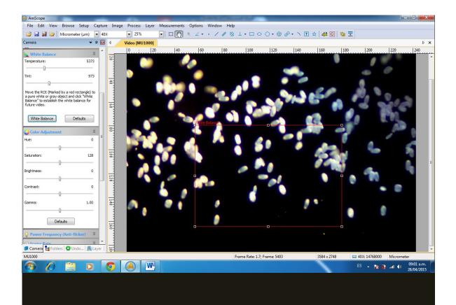
A thing to remember here is that diffraction of light is no other thing than the property of light to disperse itself when it meets an obstacle and surround it or finds a hole and passes through it; in the case of darkfield it fulfils these two characteristics because it finds a hole to pass around the opaque stop but it is also dispersed with an obstacle once you place the sample on the stage.
