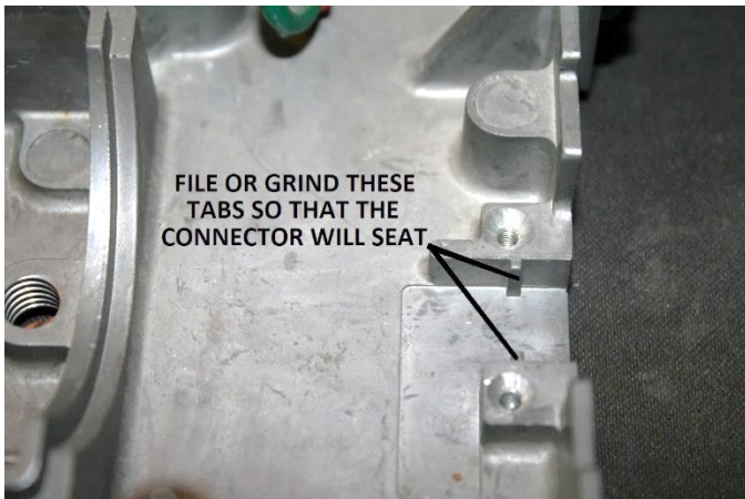
Figure 35 – File or grind casting until connector fits in recess
