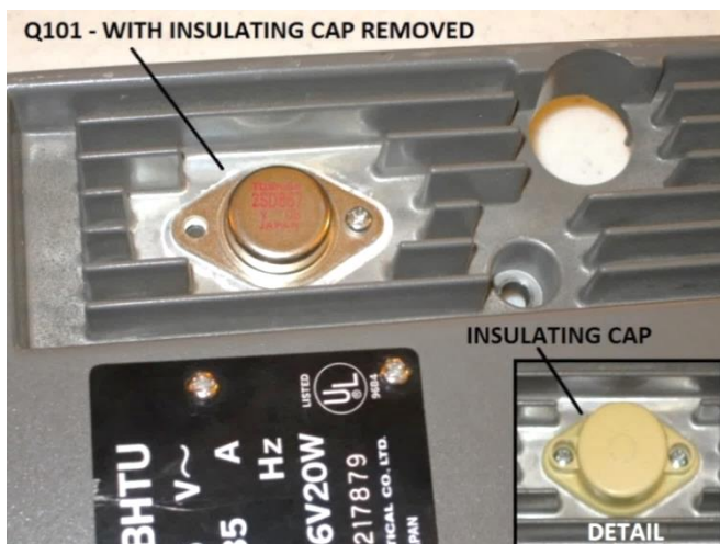
Figure 23 – 2SD867 power transistor on the bottom of the base
