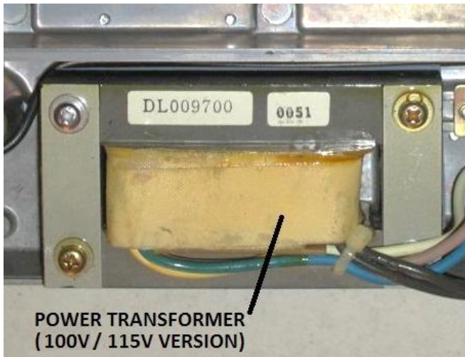
Figure 7 – Power transformer mounted onto the electrical base
