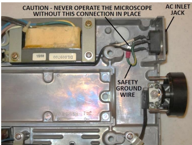
Figure 5 – Safety-ground connection for the AC inlet jack
