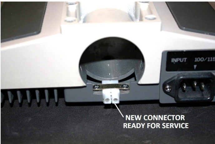
Figure 42 – Tamiya replacement ready for service
