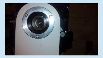
The other method that I used was to place the analyzer filter directly upon the sample and the polarizer for both methods upon the illuminator. Both methods performed very well.
