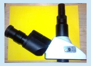
I removed the trinocular head and placed the filter on the base of its lowest optical element.
