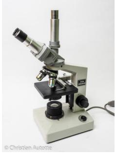
THE KYOWA WITH AN AMERICAN OPTICAL TRINOCULAR HEAD
