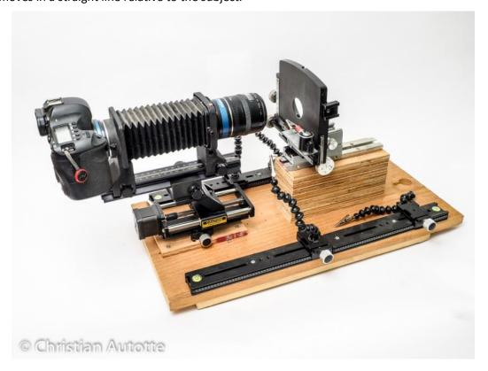
The clips that used to hold the microscope slides were removed and replaced by a thin metal plate. A small ball head was then screwed on one side of this plate, and a small crocodile clamp glued on its ¼ inch screw. The subject to be photographed is usually mounted on a pin, which is then held by the clamp. The stage control can now move the subject up and down, as well as sideways, to place it in position.
