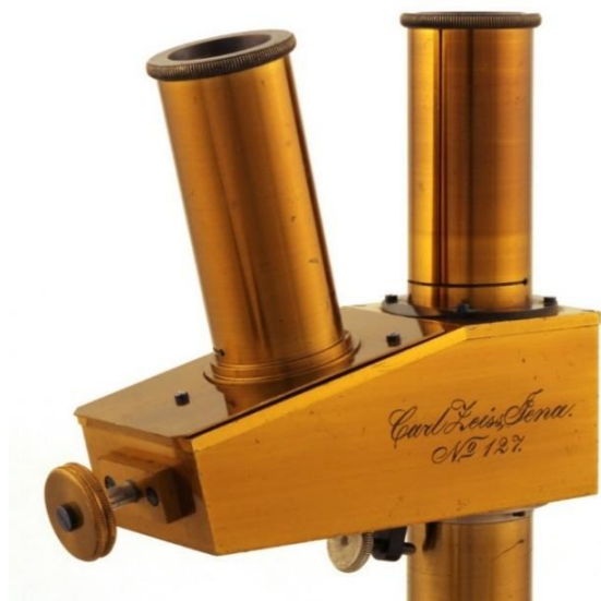
Figure 43 Abbe's Stereoscopic Eyepiece, Section [Abbe, 1880] and Photo (Courtesy Prof. Timo Mappes, http://www.musoptin.com ).
