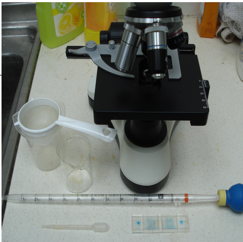
'The lab' aka the utility room with equipment ready to use. Centre front McMaster slide – more details of this below.
