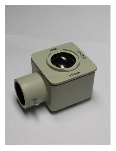
Fig. 3 OI-32 Illuminator shown without lamp assembly  $% \mathcal{A} = \mathcal{A} = \mathcal{A}$
