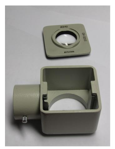
Fig. 4 Condenser plate removed
