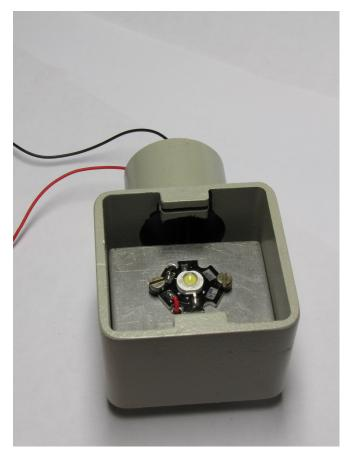
Fig. 9 LED assembly mounted and centred inside the illuminator housing
