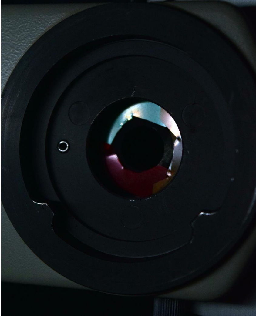
Figure 5 – Rheinberg BD filters cut from plastic shim stock (green, red and yellow in this case).
