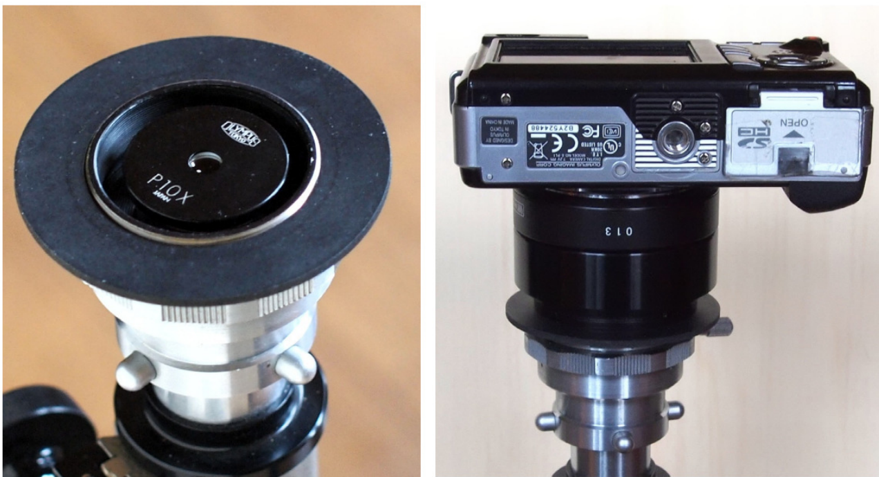
Figure 6. Using an Olympus PEN E-P1 camera on a horseshoe stand. The weight of the camera provides stability when it is positioned on a silicon gasket. This setup can also be used with a smartphone that can rest on the gasket to achieve more stability.
