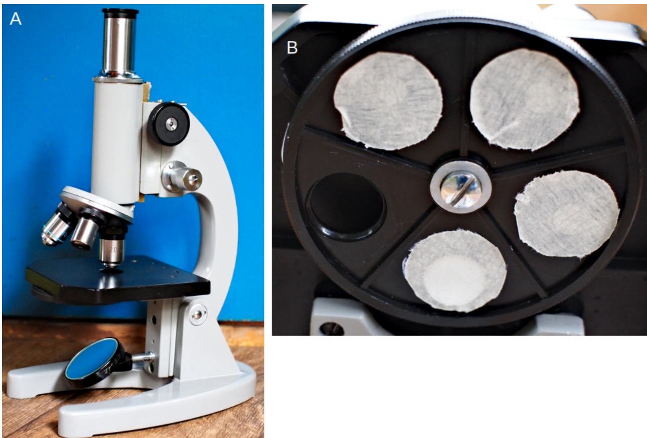
Figure 3. A: basic student microscope without substage optics (Euromex SA). B: rotating diaphragm with apertures of different sizes, 4 of them covered with Tesa tape that acts as a diffuser to optimise illumination.
