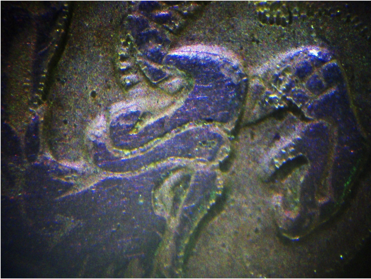
Part of the back of a Mexican one peso coin covered with a transparent tape and polarized as above 4X.
