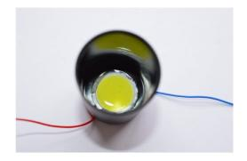
Figure 4a and b. LEDs mounted in film canisters with and without aluminium foil and diffuser disc mounted in canister lid before being re attached.
