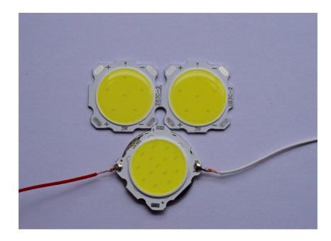
Figure 2. COB LEDs – 3 W and 7 W. Diameter of disc approximately 20mm
