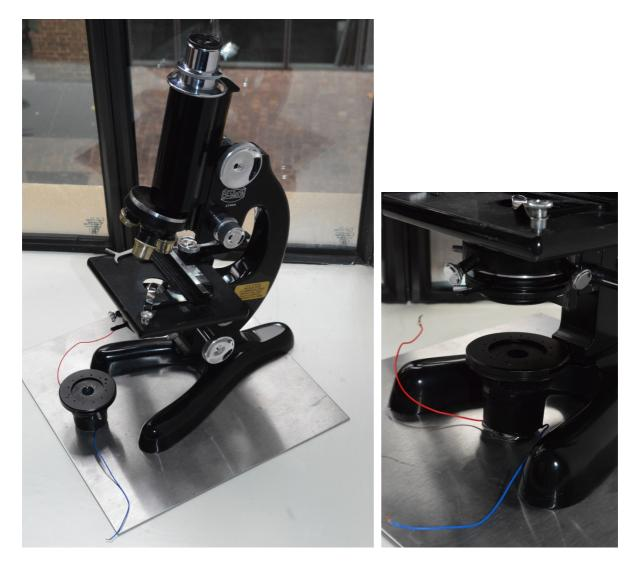
Figure 8. Beck 47 on steel sheet with magnetic Mark II illuminator being centred
