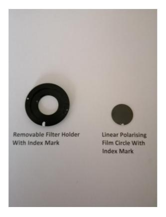
The polarising filter assembly was positioned immediately on top of the microscope substage LED lighting unit (see picture above).
