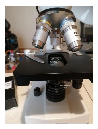
Detail showing homemade polarising filter and waveplate in position on Apex Practitioner Microscope
