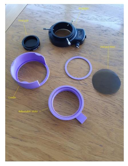
The idea being (not quite as expected as it turned out!) that light from the LED's would go down through the rotatable filter (2<sup>nd</sup> polariser) hit the specimen and bounce back up through the filter fitted into the head of the scope and thus view the specimen under polarised light.
