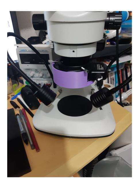
After some thinking I remembered I had a little used ringlight which I thought would give me the above light source which could somehow contain the initial polarising film. As others will know, to achieve cross polarisation requires two polar filters - one fixed the other rotatable to get extinction.
