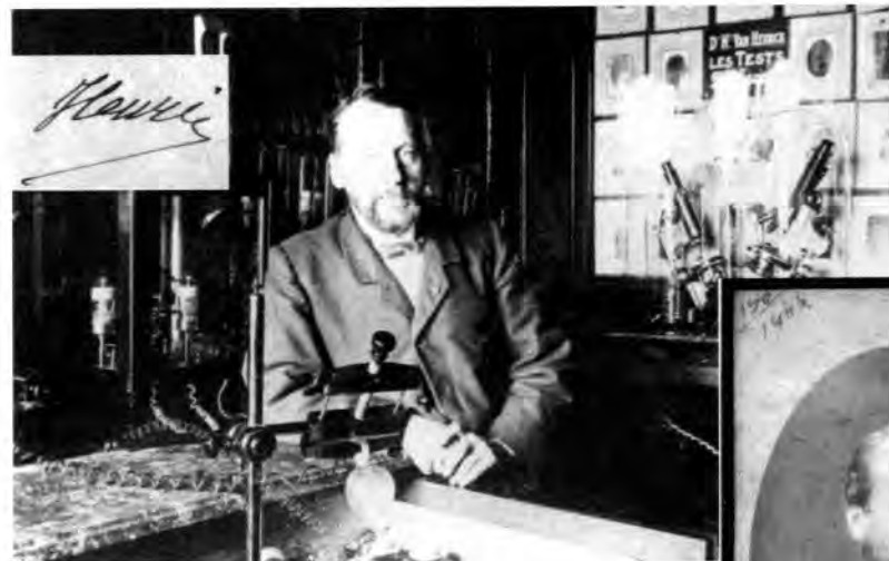
Henri in his laboratory in Antwerp. The instrument in front is an X-ray discharge tube. This apparatus was the first to be operated in Belgium, just one month after Wilhelm Conrad Roentgen's discovery in December 1895.
