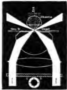
FIG. 253. REFRACTING CONDENSER WITH CENTRAL STOP (C-S) FOR DARK-FIELD ILLUMINATION.
