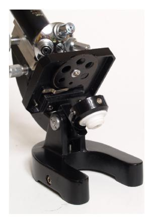
On the backside of the mirror assembly is a battery-powered lamp that turns on when the lamp is clicked into position. The batteries are mounted in the base, which also has a jack for an AC adapter.
