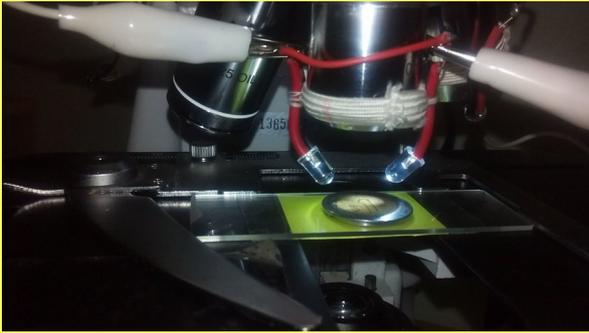
With the help of a battery box and two Cayman wires and I turn on the LEDs with a switch. Shown below is the system for only one for the two objectives.
