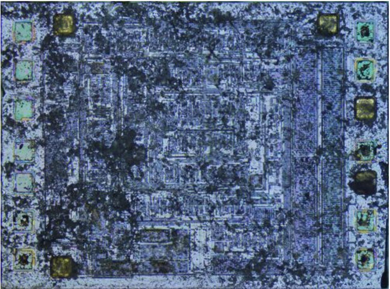
The next image is the same die after three minutes of ultrasonic cleaning. As can be seen, this is effective at removing carbonised material.
