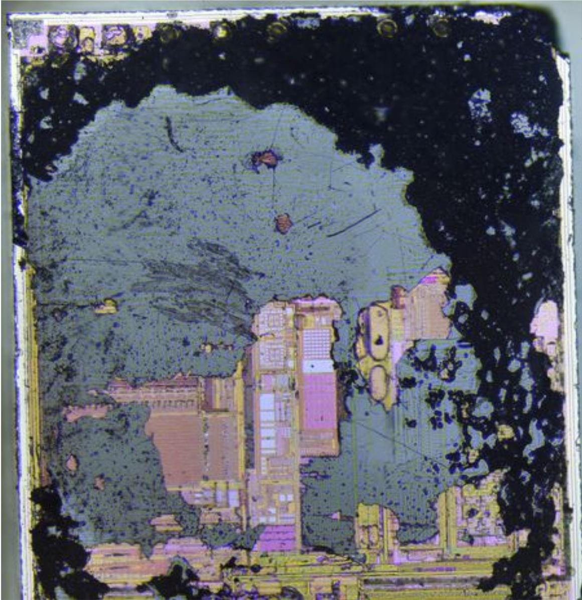
This device is one that has some sort of coating on top of the die, this is that darker black and grey areas in the photo. If I want a better view of the die, I'd try to remove this coating by burning it off and then attempting to clean the remains in an ultrasonic cleaner. In this case the die has given up enough of its secrets. In the middle of the right hand side we see this:
