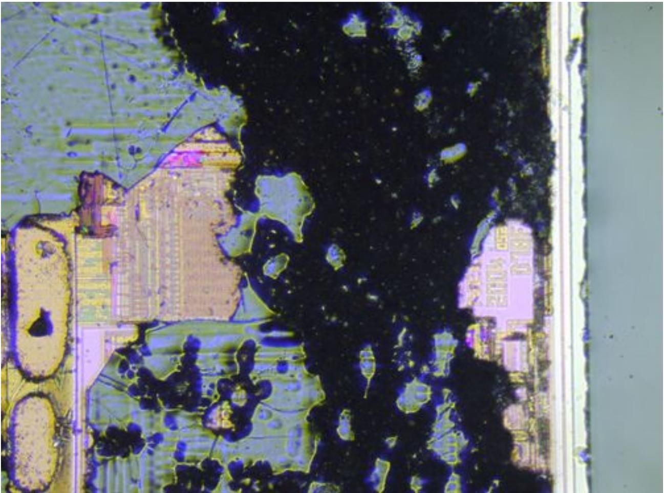
In the cleared area to the right you can see 'NEC' and D78F. This is enough to identify the device as an NEC UPD78F series microcontroller. The number of pins on the PCB that the package has narrows down the exact variation of that microcontroller. If I want to re-use the PCB I can find some devices that fit on the PCB and program them as required. A PCB that was scrap is now reusable, with a bit of work.
