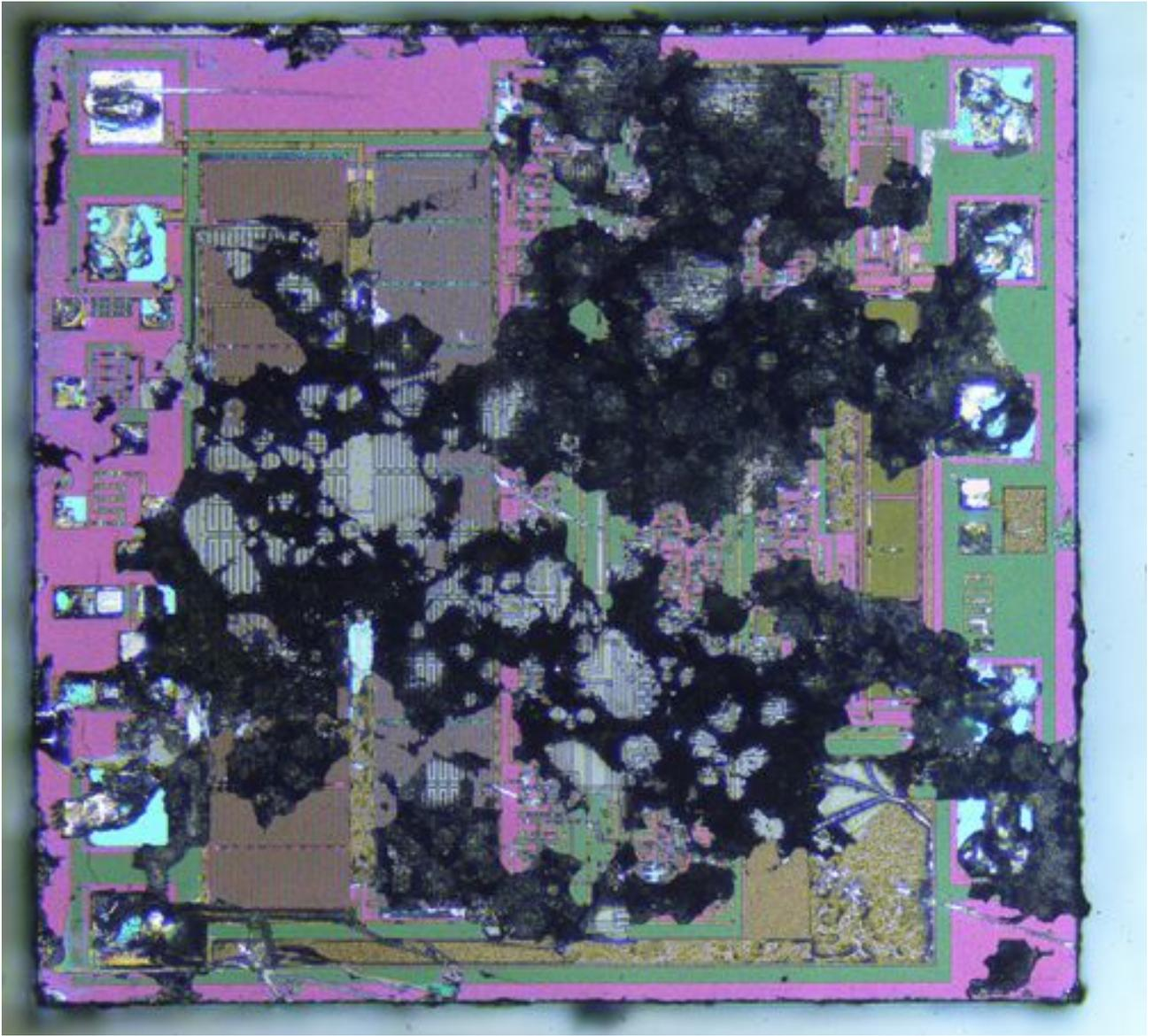
*Illustration 5: Quartz watch IC after 3 minutes of ultrasonic cleaning*
