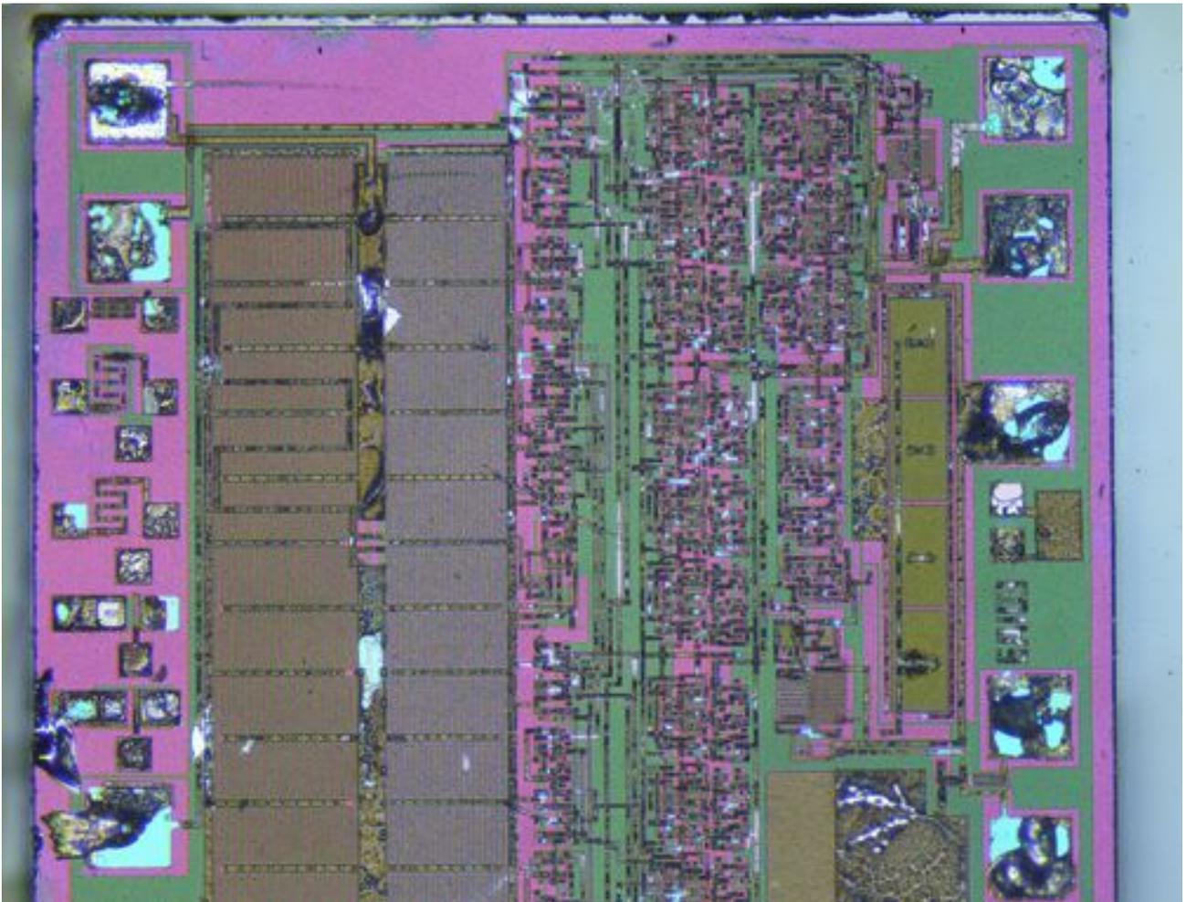
*Illustration 6: Quartz watch IC after a second heating and a further 3 minutes of ultrasonic cleaning*
