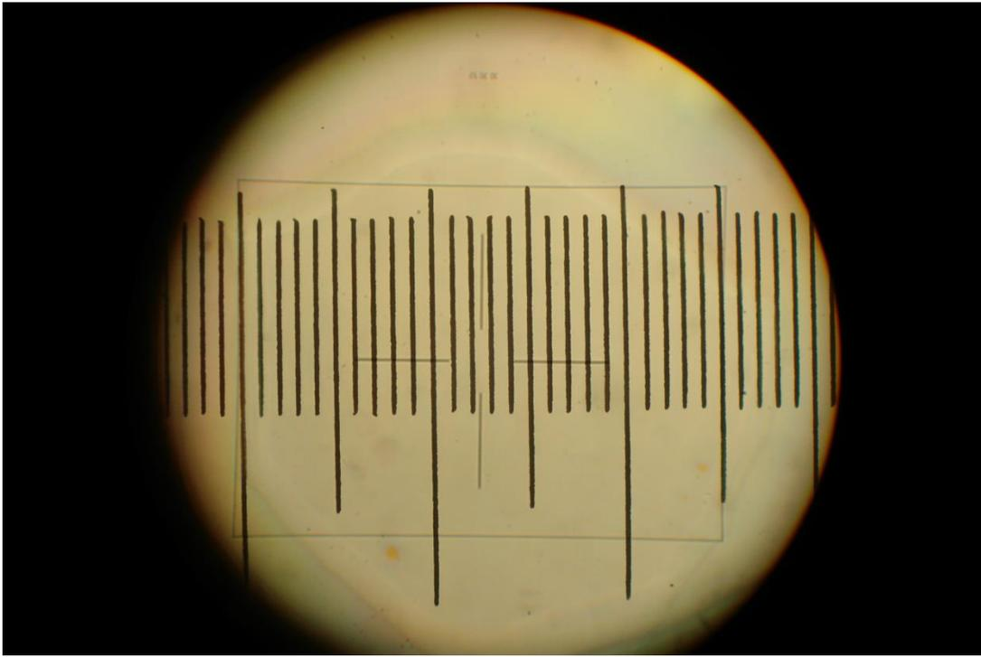
Micrometer seen through the eyepiece (frame width 0.25mm)
