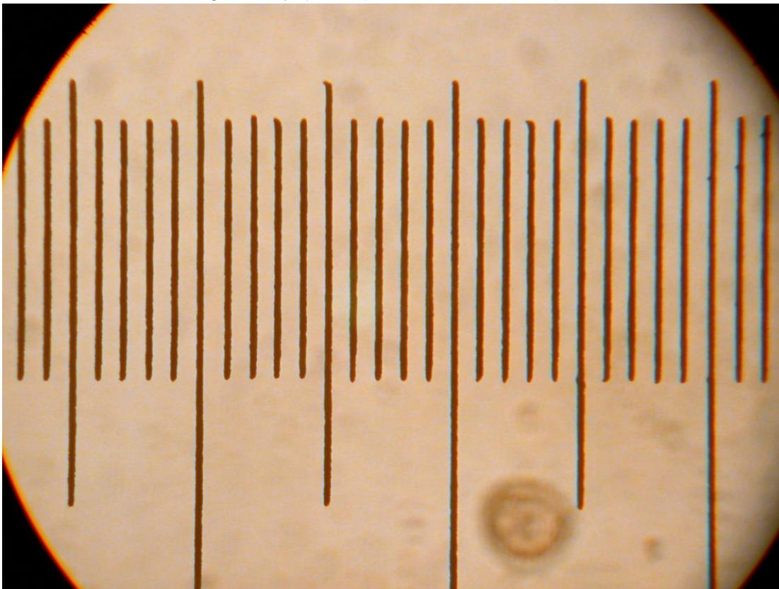
Taken by Coolpix with white balance (spot is dirt on field stop) Zeiss Planachromat 40/0.65, chromatic aberration on right probably due to some decentration in the light path. I have not figured out the cause.
