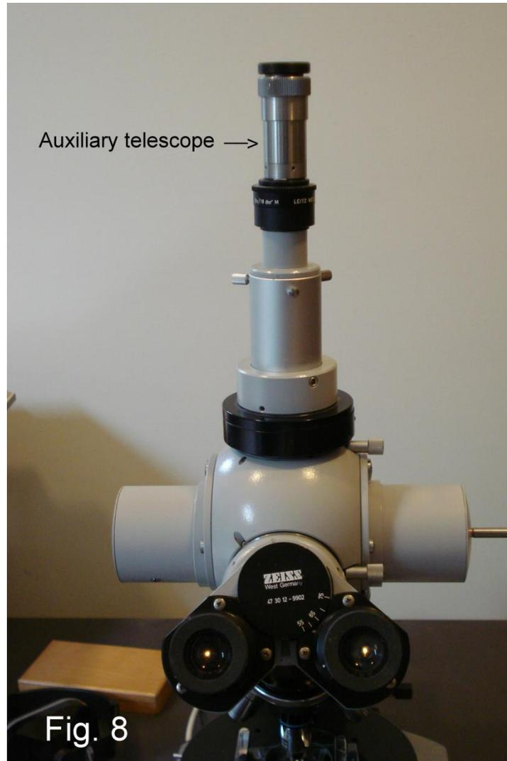
In Fig. 8 you can see the monocular, straight tube intalled on the tubehead of the Phomi. The auxiliary telescope stands on the Periplan eyepiece ready for the tube length adjustment for precise focus.
