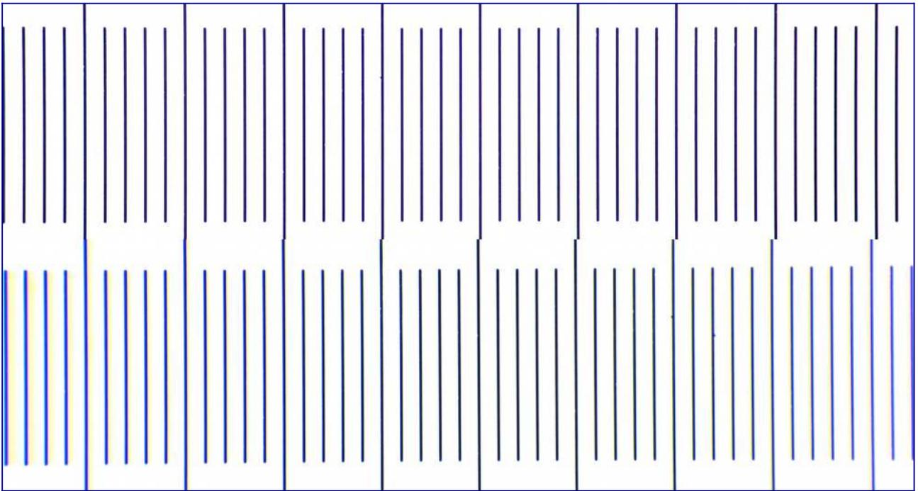
Comparison between eyepiece projection with a hybrid eyepiece (top) and a raised Kpl W10x eyepiece (bottom). Chromatic aberration is clearly visible with the normal eyepiece. Objective: CZ Plan 25/0.45.
