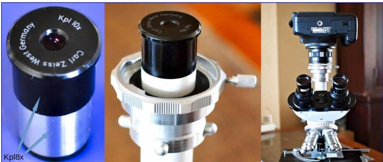
Combination of a Zeiss Kpl8x and Kpl10x eyepiece in use as a projection eyepiece with the Zeiss Standard and a Canon 600D camera. The field lens and the eye lens of a Kpl10x eyepiece were screwed onto a Kpl8x body.
