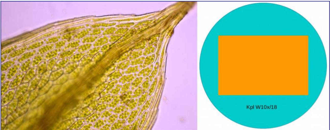
Left: a moss photographed with a Zeiss Planapo 25/0.65 and hybrid Kpl8x-Kpl10x eyepiece. Right: The orange rectangle indicates the part of the microscopic field of view that is photographed using this eyepiece and a Canon 600D camera. The circle refers to an eyepiece with a field number of 18, such as a Zeiss Kpl W10x/18 eyepiece.
