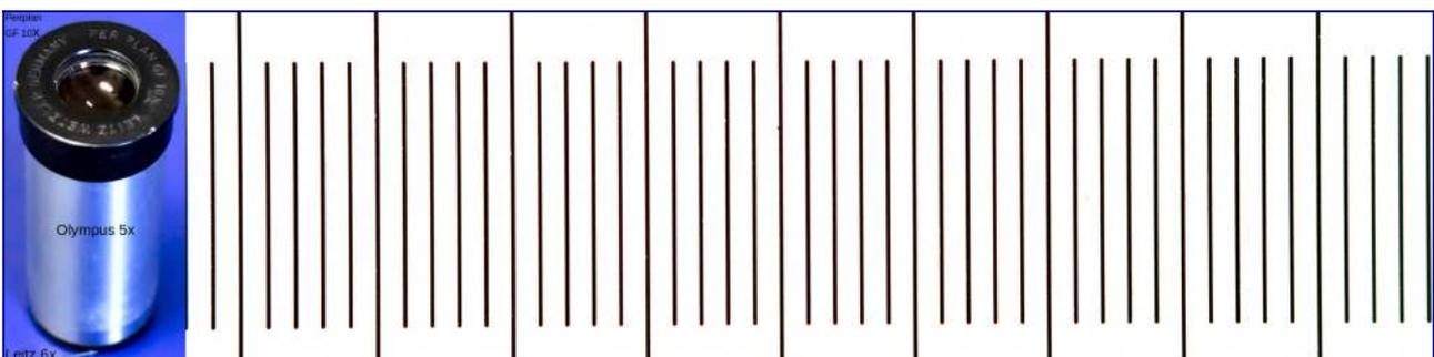
Hybrid eyepiece composed of 3 different eyepieces. Right: Stage micrometer photographed with this eyepiece and a Leitz NPL Fluotar 25/0.55 objective on the Leitz Laborlux-12.
