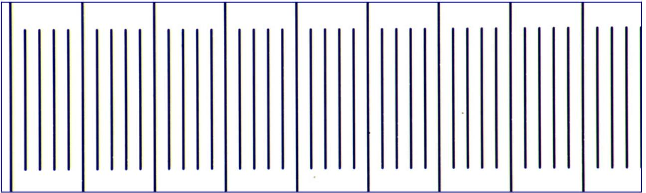
Stage micrometer photographed with 37 mm Olympus Plan 20/0.40 objective. Here, an Olympus FK2.5x projective was used in combination with the Olympus OM-Mount Photomicro' Adapter L. It is clear that a smaller part of the field of view is captured compared to the hybrid eyepiece. Camera: Canon 600D.
