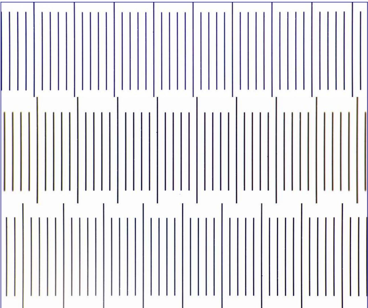
Stage micrometer photographed, from top to bottom, with Carl Zeiss Plan 25/0.45, Neofluar 25/0.60 and Planapo 25/0.65. Projection with hybrid Kpl8x-Kpl10x eyepiece.
