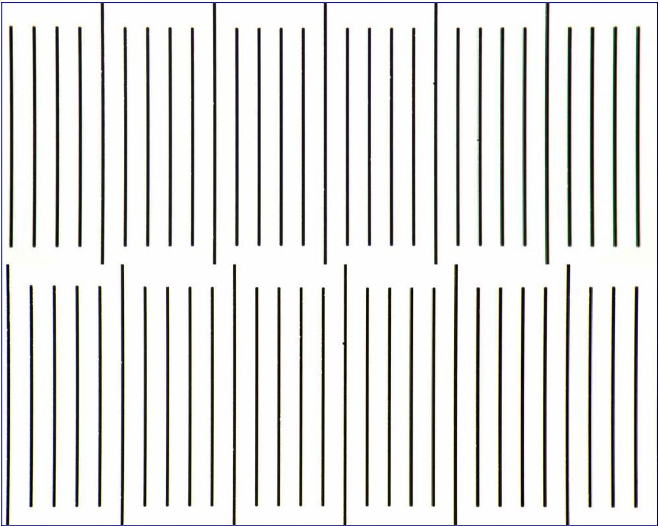
Stage micrometer photographed with Zeiss Plan 40/0.65 (top) and Zeiss Planapo 40/1.0 (bottom). Projection with hybrid Kpl8x-Kpl10x eyepiece.
