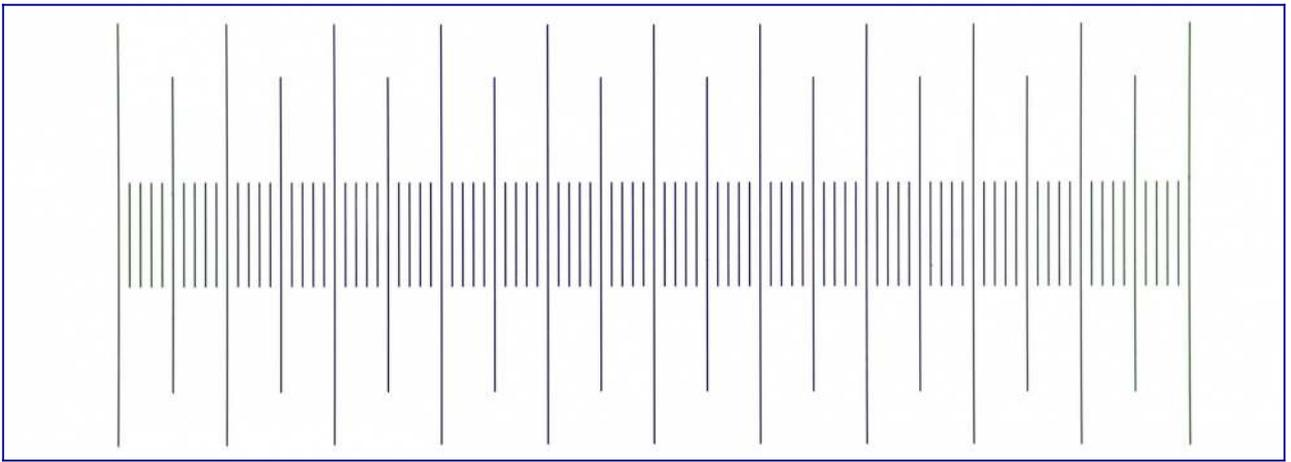
Stage micrometer photographed with a Zeiss Plan 10/0.25. Eyepiece projection with a hybrid Kpl8x-Kpl10x eyepiece.
