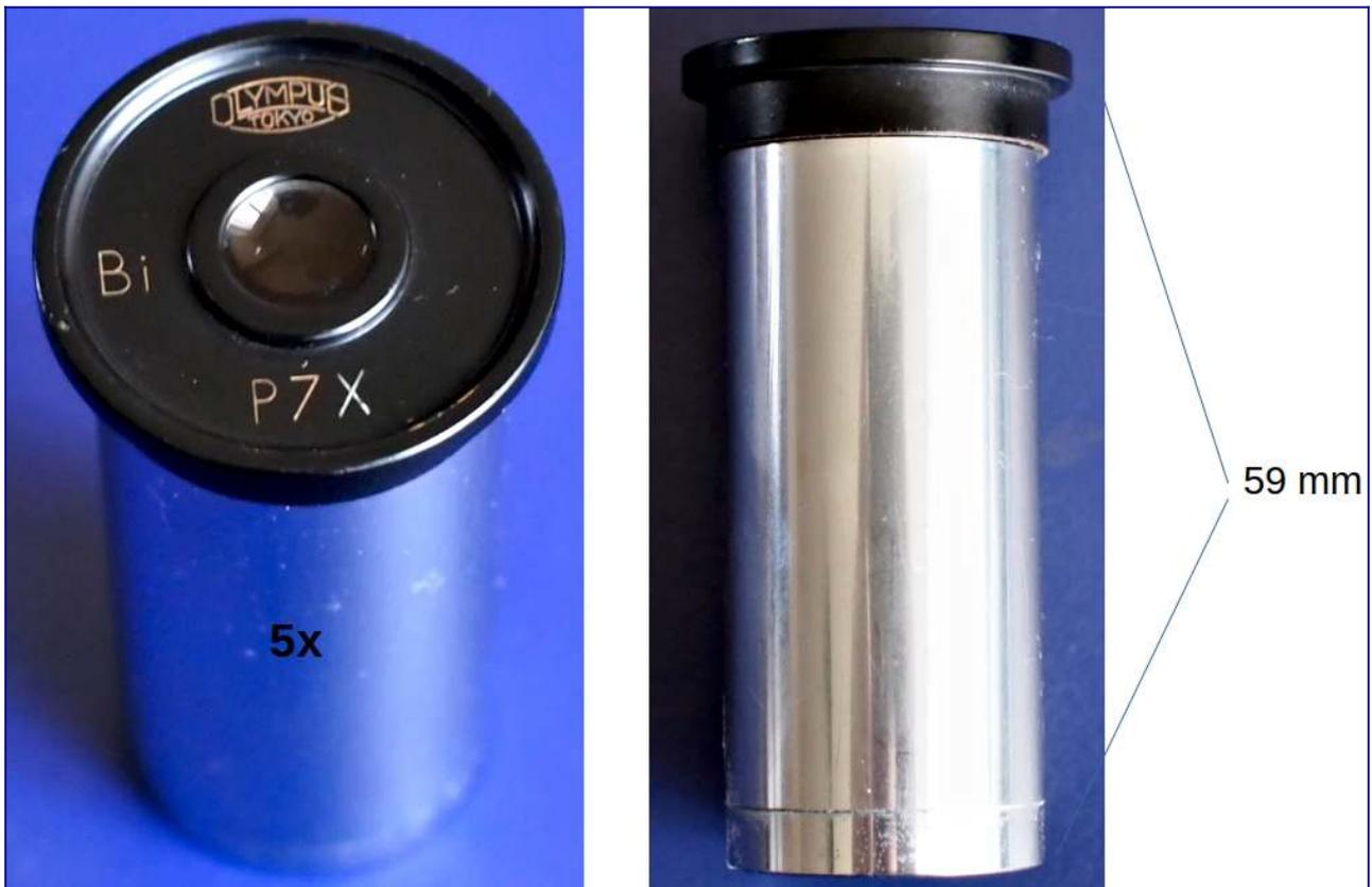
Hybrid eyepiece consisting of the lower part of an unbranded 5x eyepiece and the eye lens of an Olympus P7x eyepiece.
