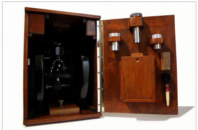
Figure 10. The Steindorff Microbe Hunter kept at Diatom Lab in its original wooden box. The monocular tube for photomicrographic or projection attachment and the oil immersion canisters are visible at the top of the lid.
