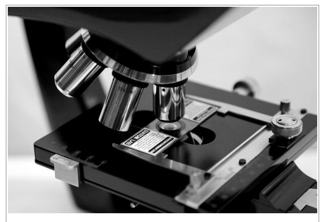
Figure 21. The Diatom Test Slide version 2.0 on the the Steindorff Microbe Hunter mechanical stage.
