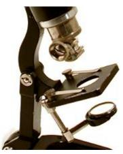
Figure 7: Detail of the flip-on objective, stage and sub and above stage mirror
