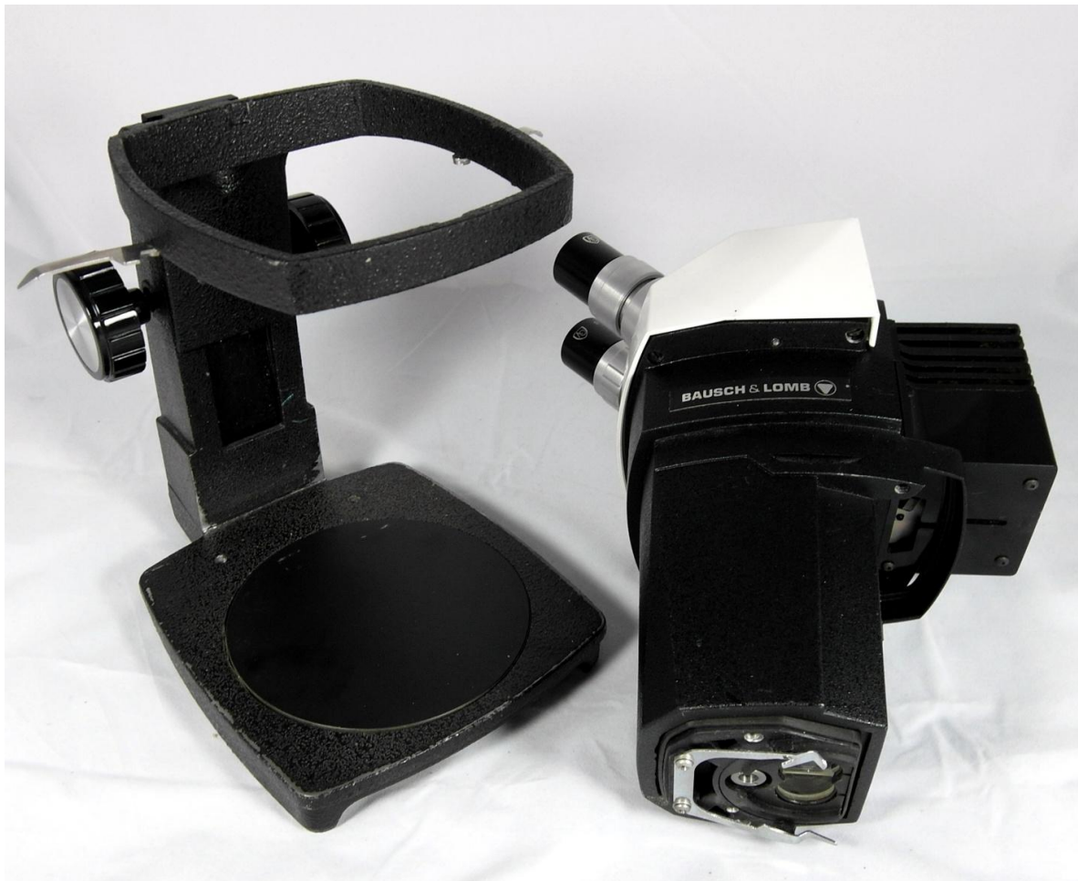
Figure 41. Bausch and Lomb StereoZoom 7, stand and microscope pod with coaxial lighting option
