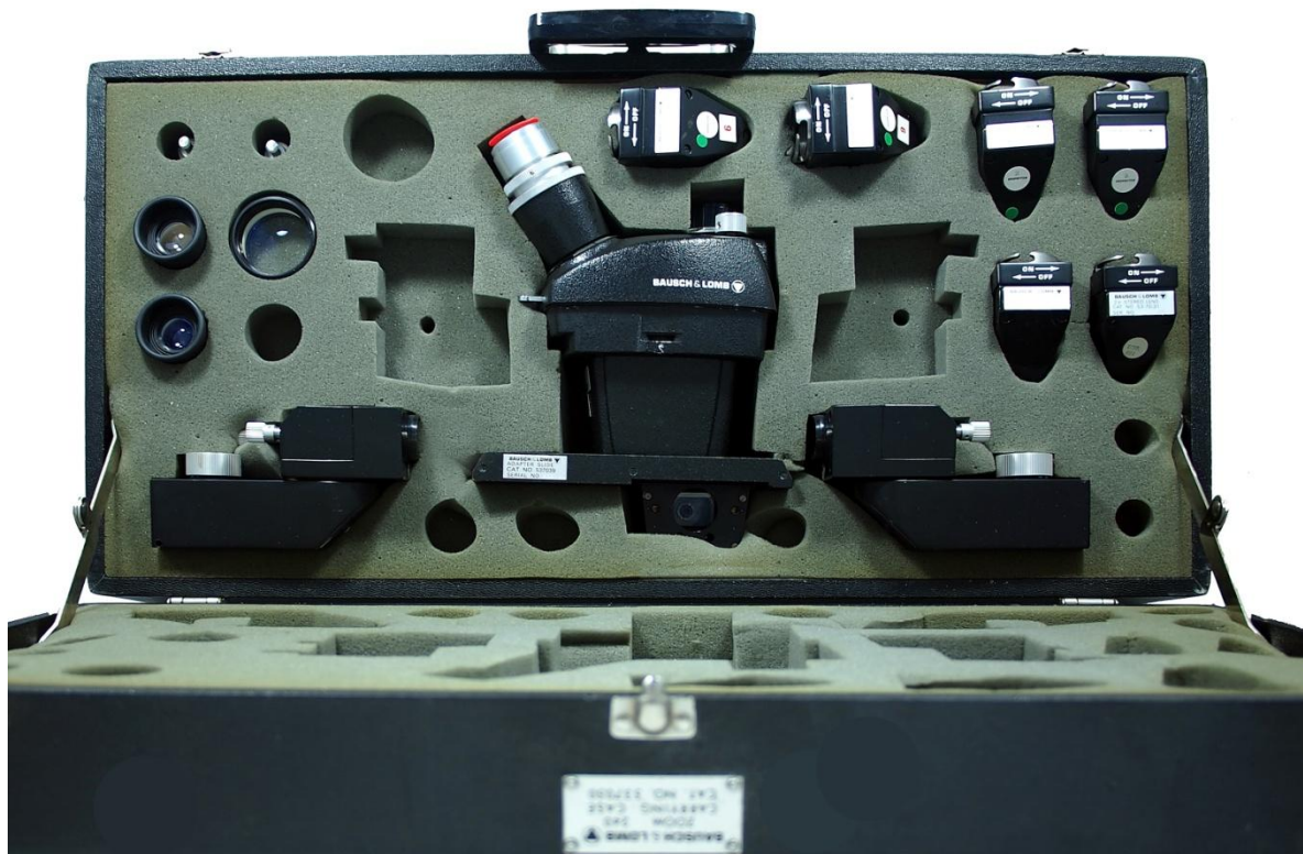
Figure 36. Bausch and Lomb 240 aerial photo interpretation stereo zoom microscope, in its laboratory storage case, with some accessories
