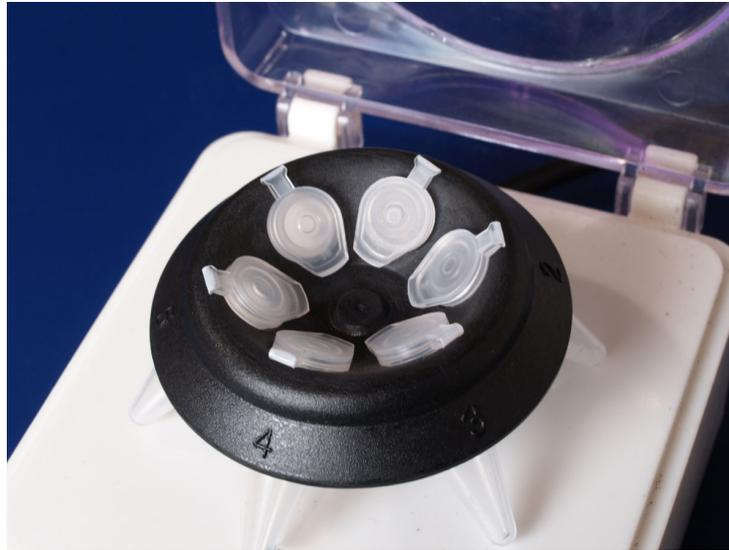
The rotor holds six 1.5 milliliter vials. You can centrifuge two or six vials at a time since the weight has to be evenly balanced. All of the vials must have equal amounts of fluid to maintain balance. If two vials are used they must be in positions opposite of each other.
