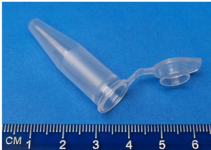
The 1.5 milliliter vials have a snap cap to prevent aerosols being created that would occur with an uncapped vial due to the Venturi Effect.
