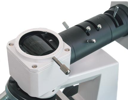
When the viewing head was replaced, it flattened the analyzer polarizing film.
