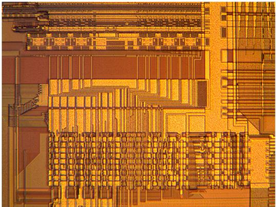
When viewed through the binocular eyepieces, the polarizer at the lamp house on the illuminator was rotated to the point where there was almost total extinction of the image. Then the exposure was adjusted in the ToupView software that supports the CMOS camera to about 0.3 seconds to compensate for the darkness of the image.
