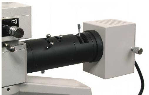
Since the East-West and North-South effectiveness is relative to the orientation of the analyzer, determining which polarizer will be the most effective could be found simply by testing each polarizer against the analyzer once it is mounted.
