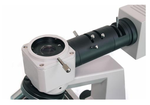
Then I simply dropped in the size-cut filter onto the top of the illuminator.
