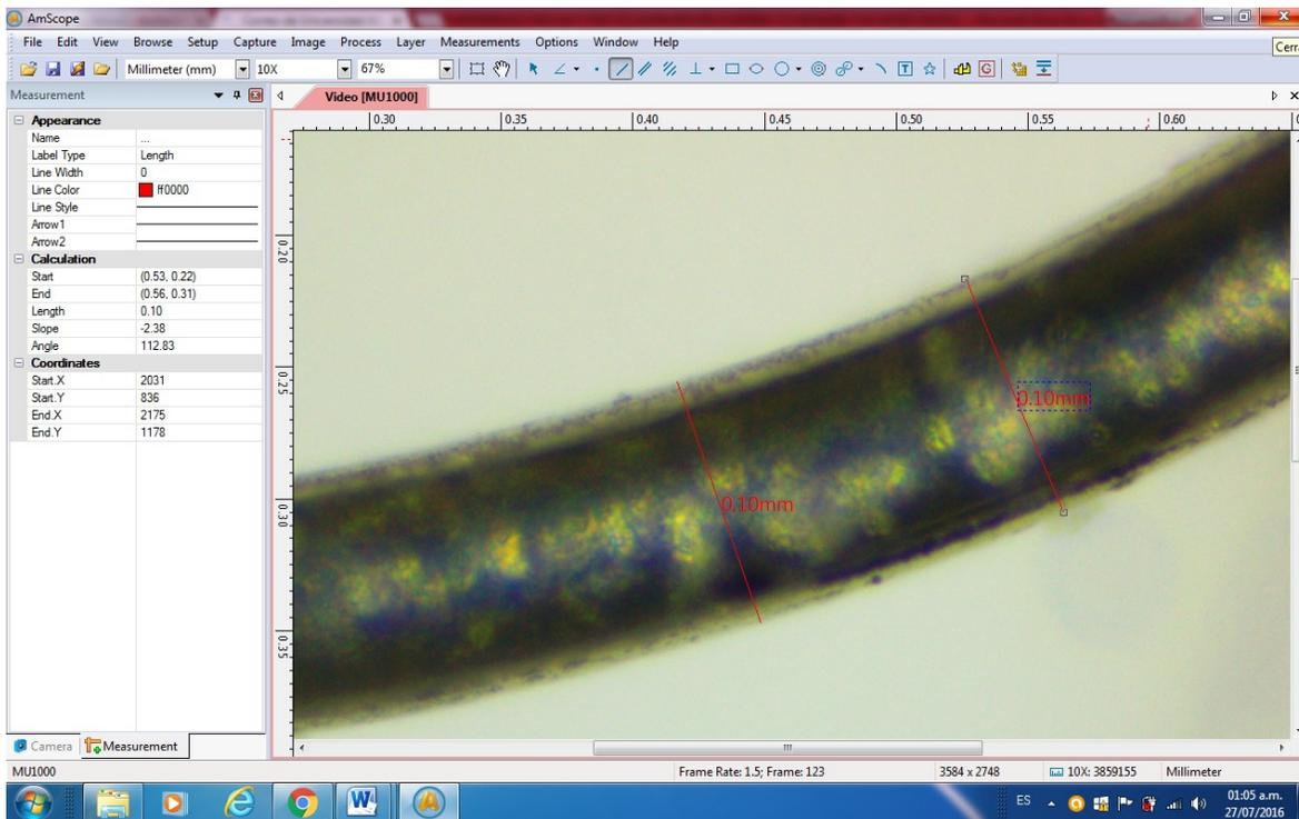
This is a very small bit of a copper wire seen with the 10x objective and 67% zoom, it is about 0.1 mm according to the image below.
