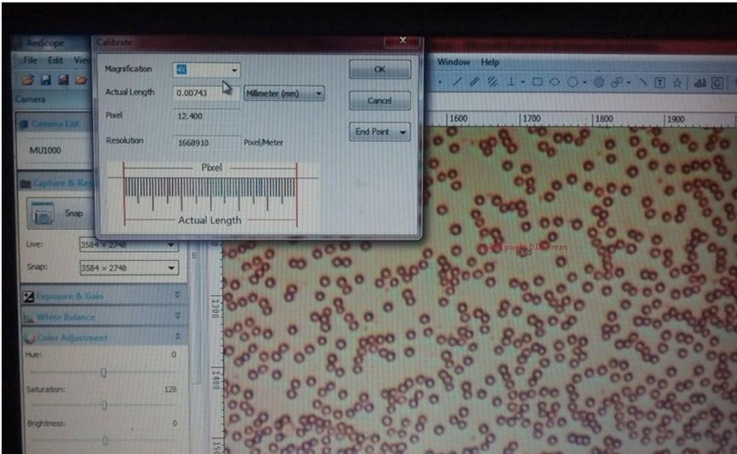
We apply the function and that is all - we have calibrated the camera for the 4x objective with a “household reference”
