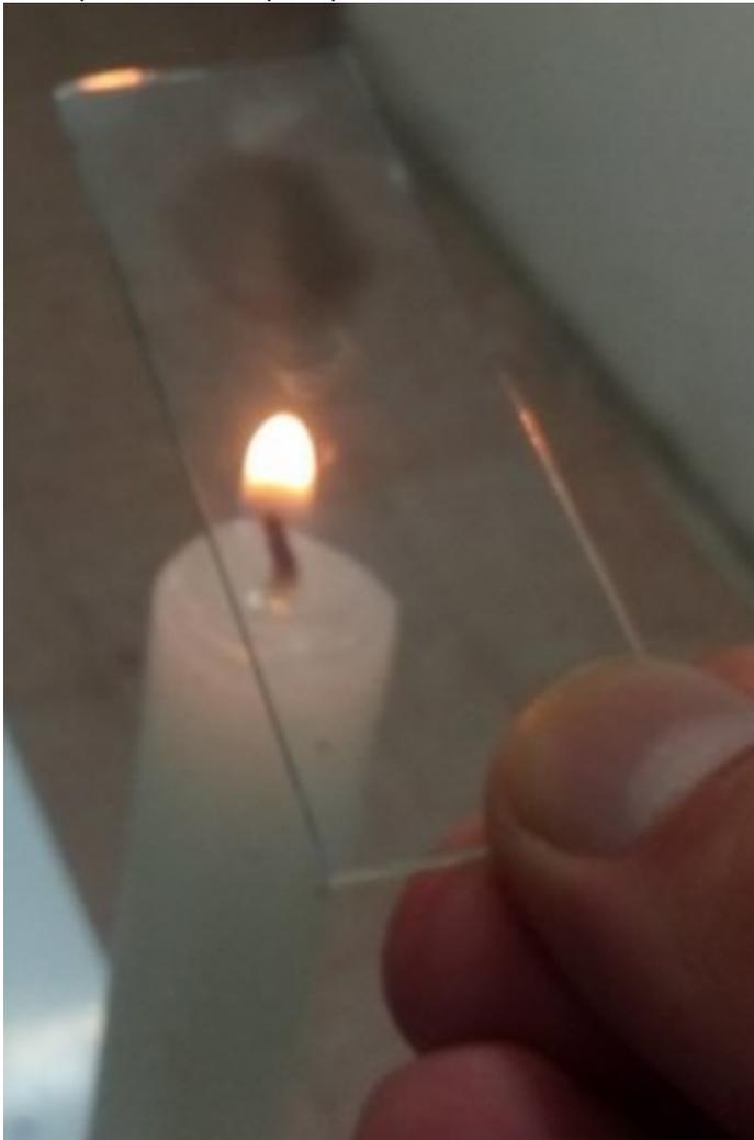
Note: Since I do not have a burner, for the moment I use a candle - obviously it is necessary to clean the soot from below the slide.
