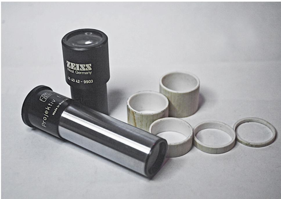
The Zeiss Projektiv  $f = 63\text{mm}$  (front), a Zeiss 10x KPL eyepiece (back) and several pieces of close fitting electrical PVC pipe cut to 2.5mm, 5mm, 10mm 15mm and 20mm used to *lift* the eyepiece by lengthening its shoulder. Varying the height over and above the initial *lift* that enables it to project a real image alters the magnification ratio.
