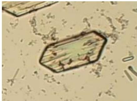
Figure 10: Picture of a single silver acetate crystal
