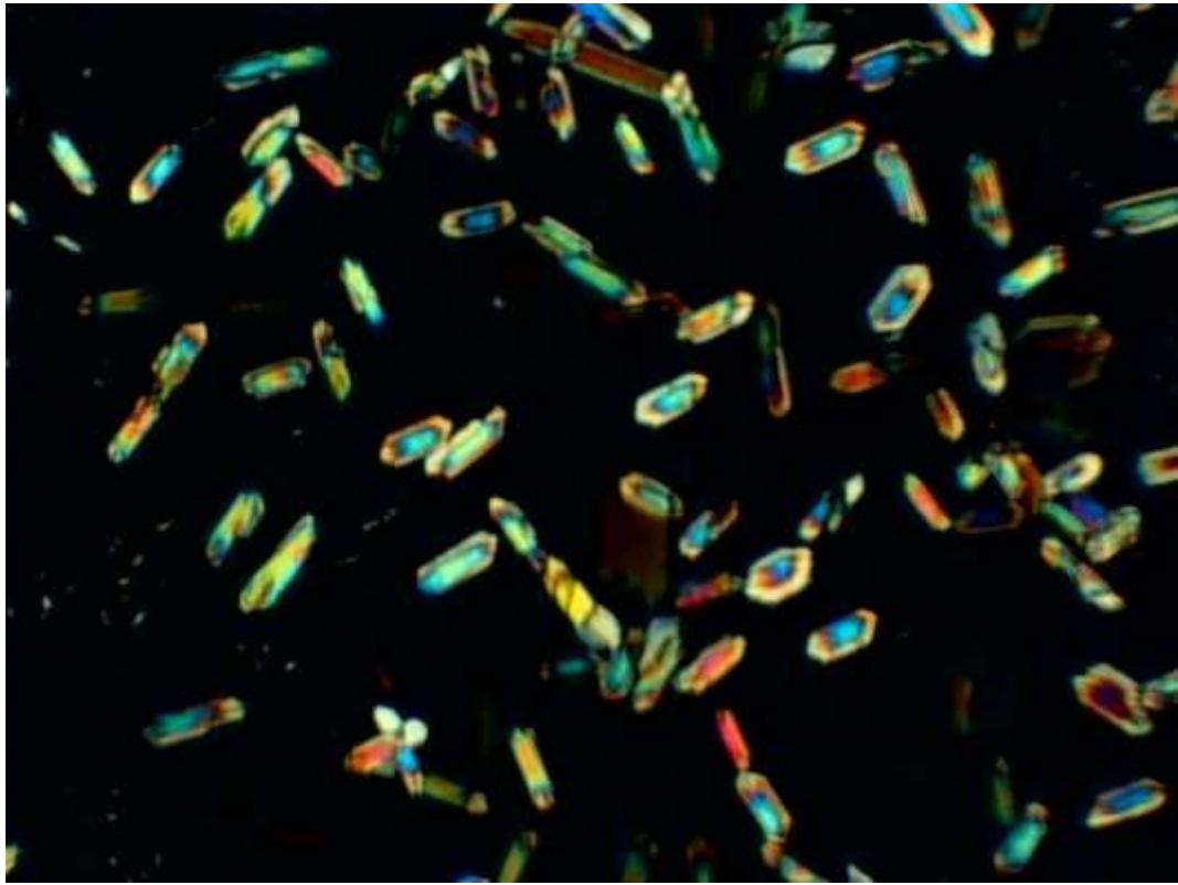
Figure 7: Silver acetate crystals in polarized light (obj. 10 x)
