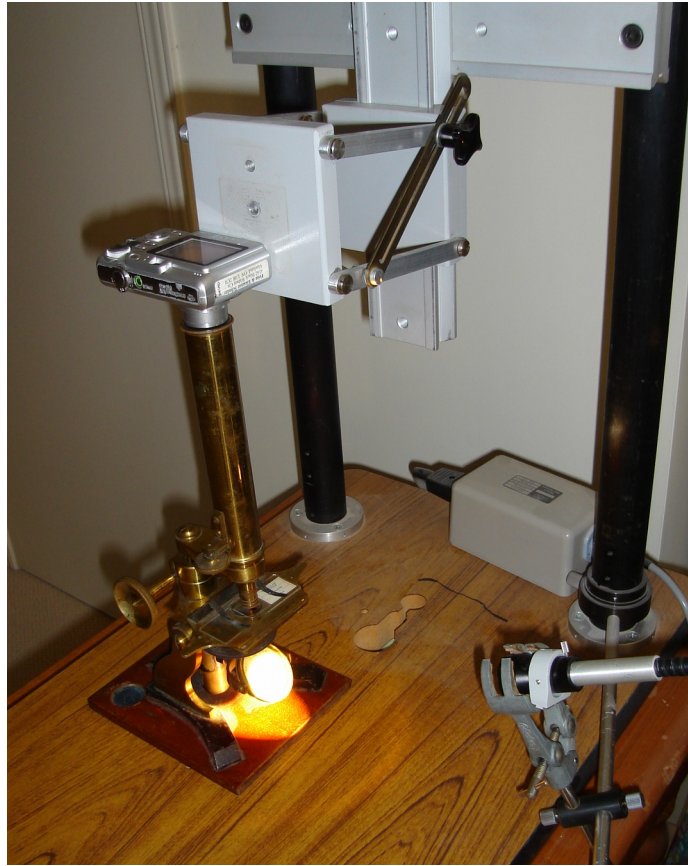
My set-up for taking photomicrographs on home-made macro-stand
