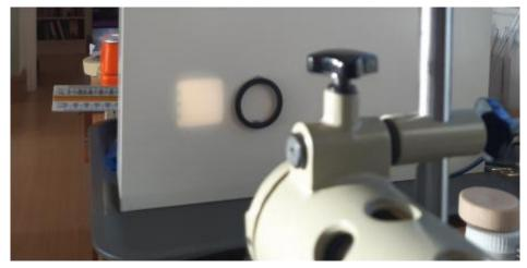
The black ring Blu Tacked into place in each photograph is 35mm outside 28mm inside diameter, so similar to the filter holder on many substage condensers. Better for Köhler illumination I think.
