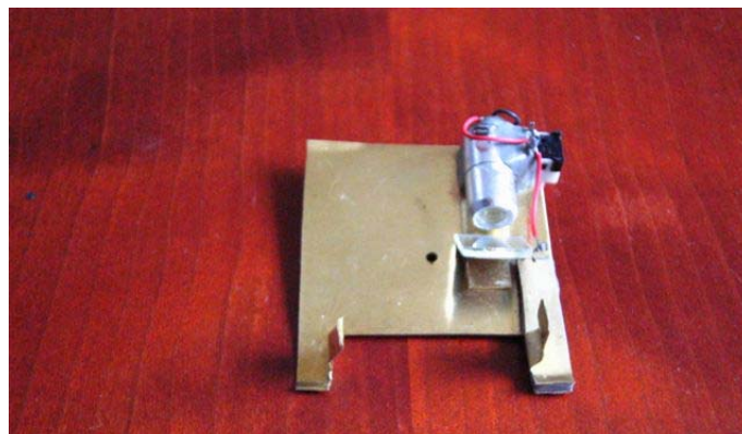
Illumination system in the chassis
